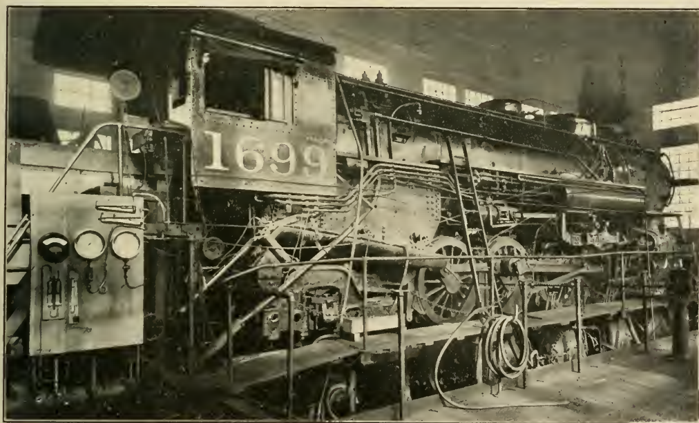
Three-Cylinder Locomotive of the Missouri Pacific Railroad on the Test Plant of the Pennsylvania System at Altoona, Pa.
